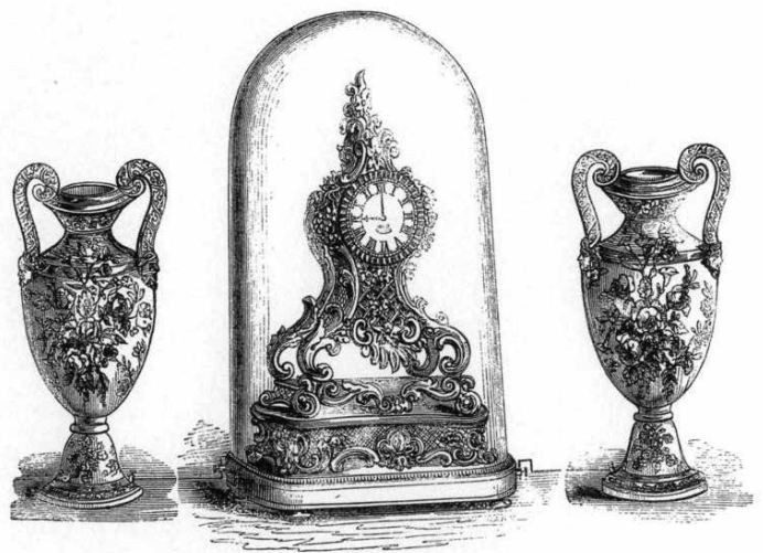
Fig.8: The vases are the earth batteries containing the zinc and copper plates as an alternative to placing them in the ground. This arrangement was especially useful for clocks intended for use upstairs. From: A Bain, A short history of the electric clocks (1852).
